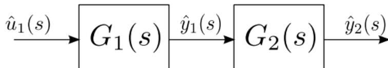
$$\begin{aligned}\hat{y}_2(s) &= G_2(s)\hat{y}_1(s) \\ &= G_2(s)G_1(s)\hat{u}_1(s)\end{aligned}$$
