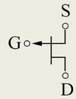
$$g_m = \left[ \frac{\partial I_D}{\partial V_{GS}} \right]_{V_{DSconst}} = -\frac{2}{V_P} \sqrt{I_{DSS} \cdot I_{Drepose}}$$
