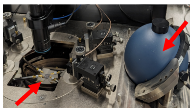
Fig. 2 The measurement apparatus used to carry out on-wafer measurements, showing the piece of wafer containing the VCSELs (left arrow) and the fibre-coupled integrating sphere (right arrow) that gathers the light output.
