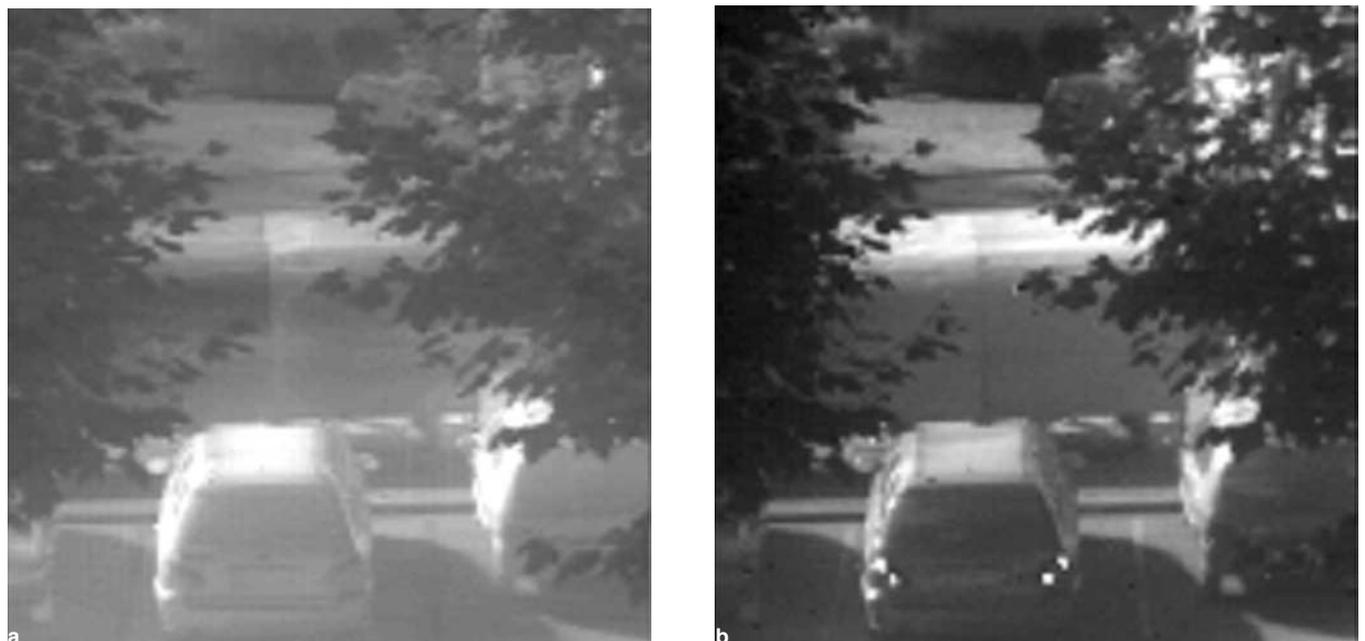
Fig. 11. Example of a dual-band image showing a car in a parking lot with back lights on. (a) longest wavelength image (MWIR2) and (b) short wavelength (MWIR1) image. The device used is grown on CdTe/Ge (2566).
