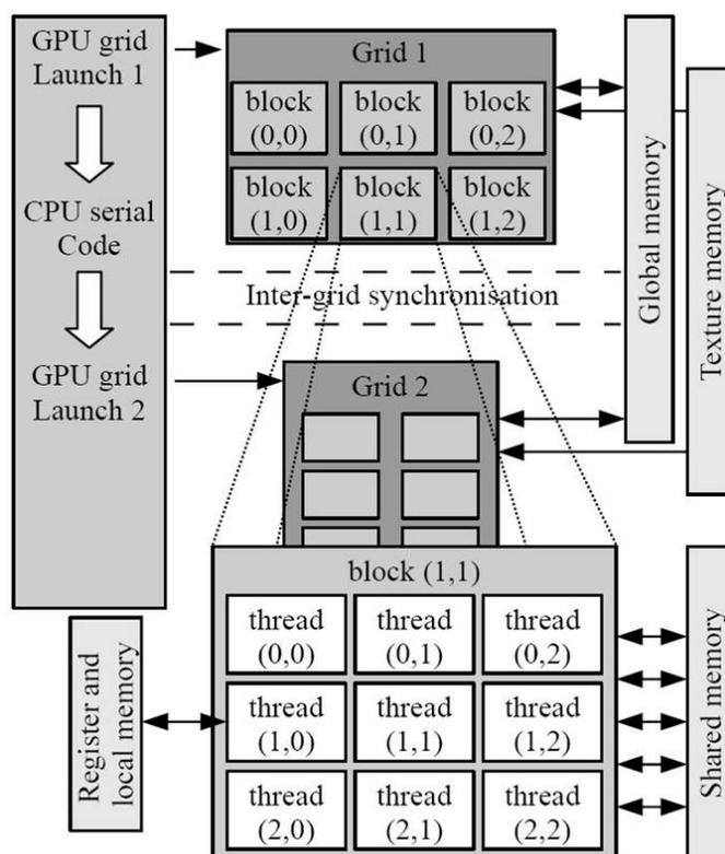
Figure 1. Thread and memory hierarchy in GPU
