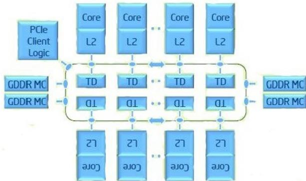
Figure 2. MIC microarchitecture
