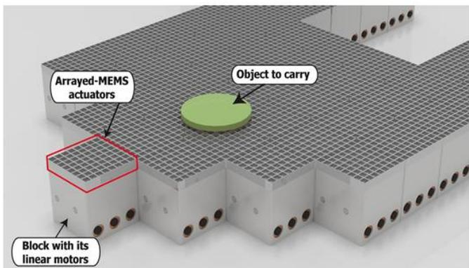
Figure 6. The Smart-Blocks conveyor
