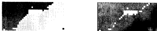
Figure 2: False matches at the border of a rock: disparity image (left), and correlated pixels (right).
