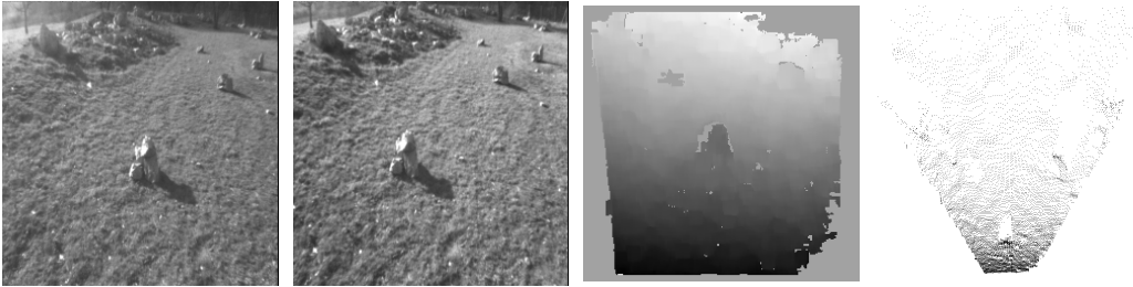
Figure 4: Pixel-based stereovision. From left to right: a stereoscopic image pair acquired with Lama, the disparity image produced by the correlation algorithm, and a top view of the corresponding 3D image.
