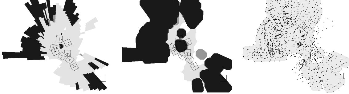
Figure 5. The model structuration procedure. From left to right : a terrain model resulting from the fusion of 8 classified laser images ; the same model after constrained zones growing, and the nodes of the connection graph defined by the region segmentation
