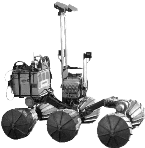
Figure 8: The robot Lama, a Marsokhod robot built by VNIITransmach and equipped at LAAS
