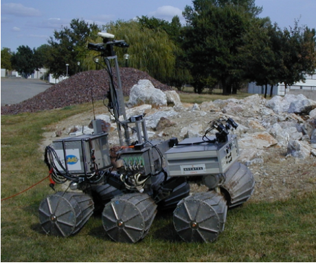
Figure 2: The robot Lama used for the experiment (the panoramic camera can not be seen here - it was mounted on top of the mast, near the white GPS antenna). The numbers indicating the position of some images.
