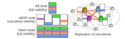
Fig. 5. The routing table is split between the n = 4 nodes of the overlay
