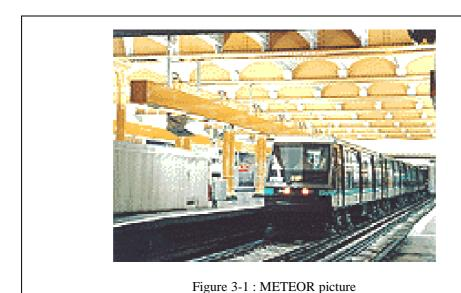
In October 1991, RATP started the METEOR project. METEOR is a new generation underground railway whose main feature is its fully automated operation. The length of the line is 19,6 km with 20 stations and will transport 40 000 passengers/hour.
