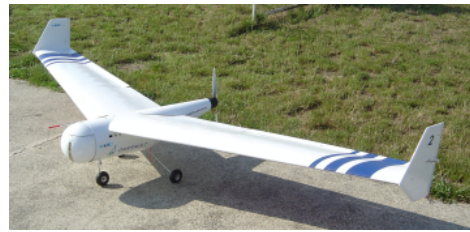
Fig. 8. The UAV Lhasa (3.0 m wingspan, 6.0 kg total)
