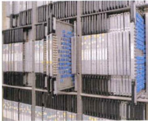
The ILLIAC IV supercomputer led its field in 1966 as a parallel computing machine. This computer was only ever quarter finished, but took eleven years to build at nearly four times the original estimated cost. Image courtesy of Steve Jurvetson
