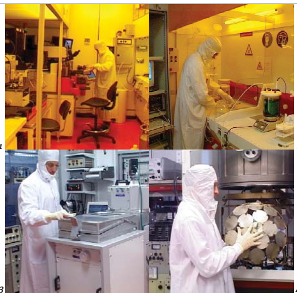
1- Photolithography room 2- Electrochemical deposition benches 3- Silicon deep etching machines 4- Metals deposition systems
