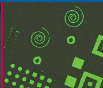
imprinted in a curable material, right side: micrometric patterns of fluorescent antibodies deposited by μcontact Printing.
