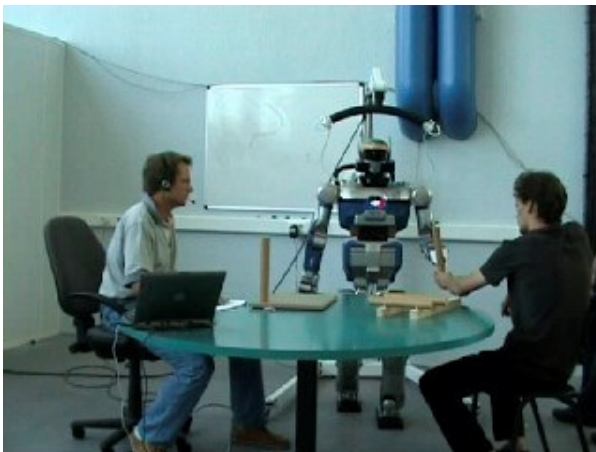
Fig. 3B. After the “prepare” command, HRP-2 has left hand in grasping position. User2 positions the leg in the gripper, and User1 issues the “close left” command. HRP-2 closes left hand to grasp the leg.
