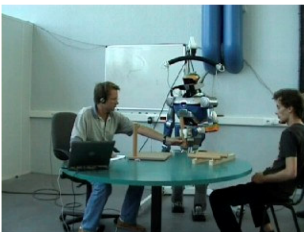
Fig. 3C. After the “give it to me” command, HRP-2 rotates waist towards user1 with left hand in giving position. User1 prepares to take the object after issuing “left open” command..
