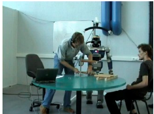
Fig. 3E After the “right close” command, HRP-2 has the table held securely in its right hand, allowing User1 to use both hands to attach the leg to the table.
