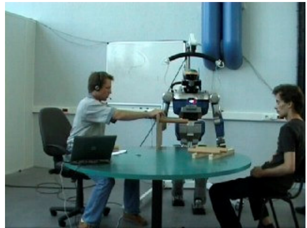
Fig. 3D. After the “hold” command, HRP-2 has right hand raised and open, ready to hold the table surface in place. User1 prepares to position the table top in the robot’s open right hand;.
