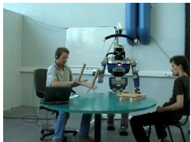
Fig. 3F. After the “open right” command, HRP-2 releases the table and User1 takes the table. At this point, the OK command is given, and the sequence is stored as a macro. User1 then invokes this for the third and fourth legs with the command “macro.”
