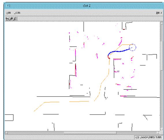
Figure 5: A navigation task : the planned path and its execution.
