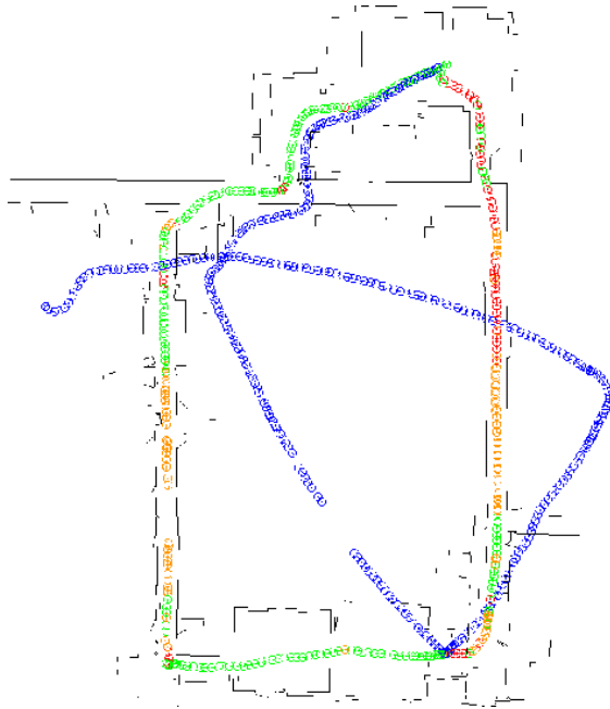
Figure 4: Comparison of position estimation obtained from XR4000 odometry alone (dark circles) and from the SEGLOC module (gray circles).
