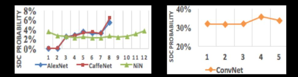
1.Layers 1&2 have lower SDC probabilities in AlexNet and CaffeNet
