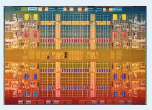
Intel Mehalem-EX, 2009 8 cores, 24MB cache 2.3B transistors
