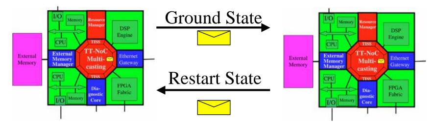
Component sends its ground state regularly to the ground-state monitor Ground state monitor performs error detection and restart with a state-estimated restart state
