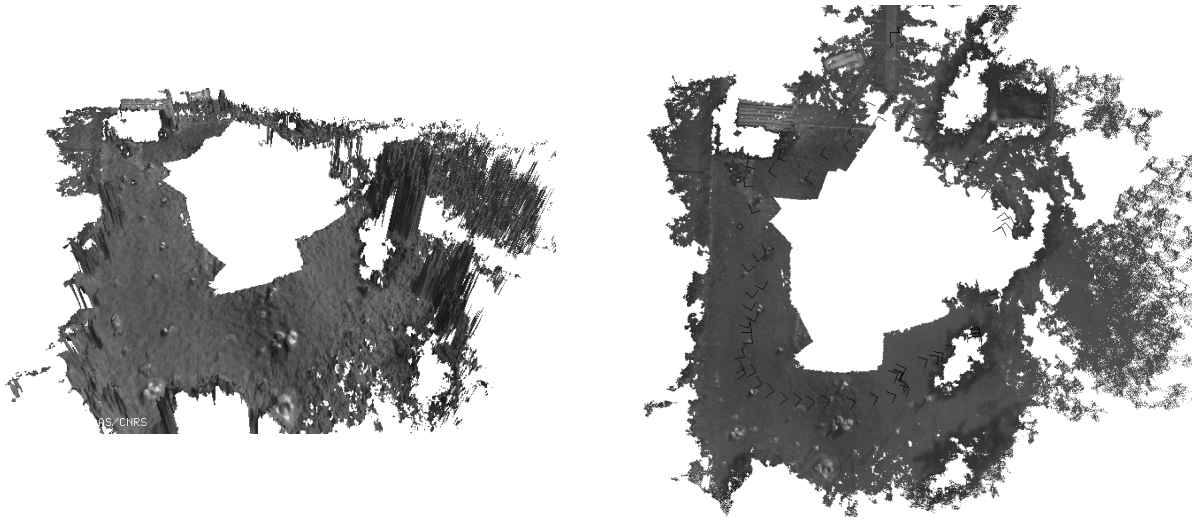
Fig. 12: Final digital elevation map produced with the 80 stereovision images corresponding to the third trajectory of figure 1. The overall position estimation error can be seen on top of the right image, where the first and the last images overlap (see the calibration frame). The absolute translation error is about 1m at the end of the trajectory.
