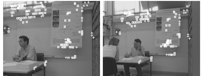
Figure 9: Matching with scale and view point change, and moving elements in the scene. 73.9% of the matches are valid, computation time is 0.6s.
