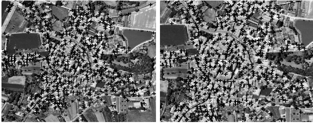
Figure 1: Interest points detected on an aerial image pair (black “+” junctions). The transformation between the images is here a 1.3 scale change, and repeatability is 63%.
