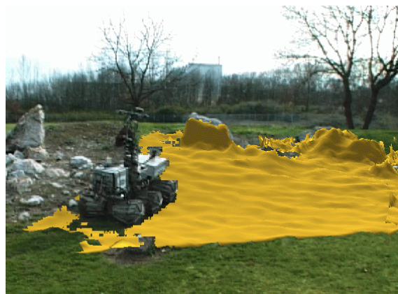
Figure 1: The robot Lama during an autonomous rough terrain traverse. Here, the digital elevation map built during the traverse is surimposed on the image.
