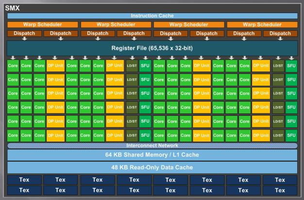
Figure 2.8. SM architecture (modified)
