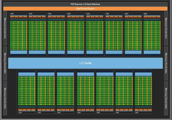
Figure 2.7 NVIDIA Kepler GK110 architecture
