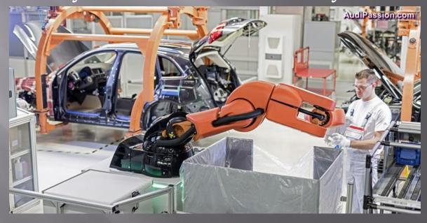
Fig.1.5 Collaboration of man & robot AUDI, Ingolstadt, Germany Workshop Artificial Intelligence, LAAS-
