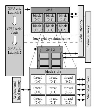
Figure 2. Thread and memory hierarchy in GPUs
